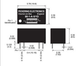
Schematics are shown from UNDERNEATH the relay.
