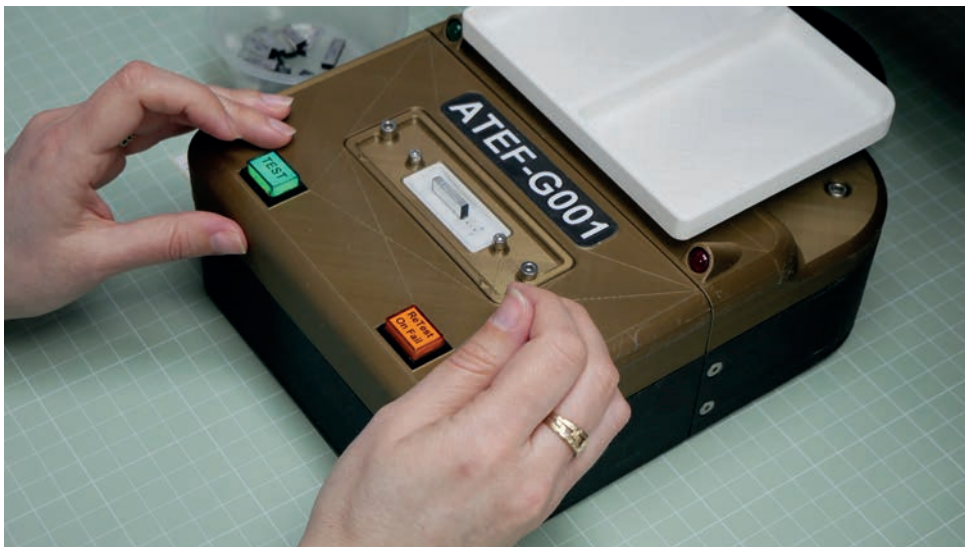
Fig. 4.1 - A Pickering ATE System for Testing Reed Relays
