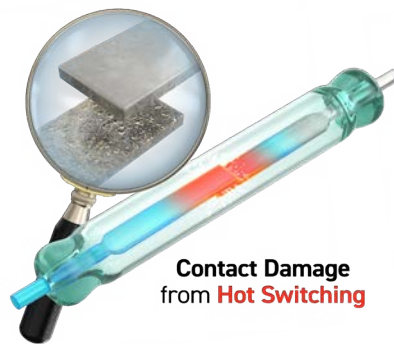
Fig. 8.1 - Hot Switching Damage
