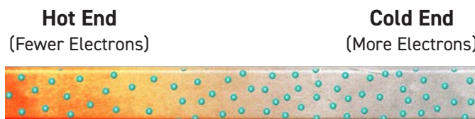
Fig. 5.4 - Thermal EMF Across a Conductor
